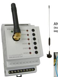
6 x 8A switching receiver with 3 normally open contacts and 3 normally closed and/or normally open contacts.
