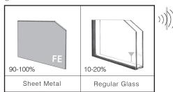
Signal range testing is crucial as modern building materials can contain aluminium lined plasterboard, aluminium lined polystyrene insulation and energy saving glass with a metal oxide coating.
