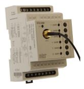
Remove original internal antenna supplied and fit the AN-E external antenna.
