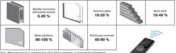
Note: Where the signal is reduced through building materials or elements the ClickSmart repeater (RFRP-20/B) can be used to help increase the signal range and also assist in bypassing elements causing signal reduction.
