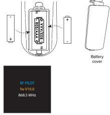
The memory has an independent power supply. Any custom adjustment (except for time and date) will remain. After inserting the batteries, the RF Pilot name and the firmware version will appear on the initial screen as shown above. To set the Date and Time elements see page 14.
