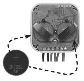
3. Install batteries ensuring correct polarity
