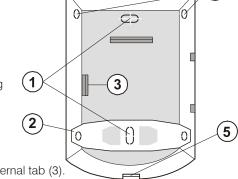
C. Punch screw holes through the rear plastic cover - for a flat wall (1) or for 45° (corner) mounting (4).
